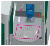
Fixture dimensions: 700 x 798 x 1000 mm (W x D x H)
