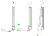
**1.** Dismantle the according protection flaps of the SPEED-Bus slot with a screw driver (open and pull down).
