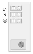
The power supply is provided with AC voltage by means of the input slot.
