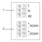
For the cabling of power supplys a green plug with CageClamp technology is deployed.
