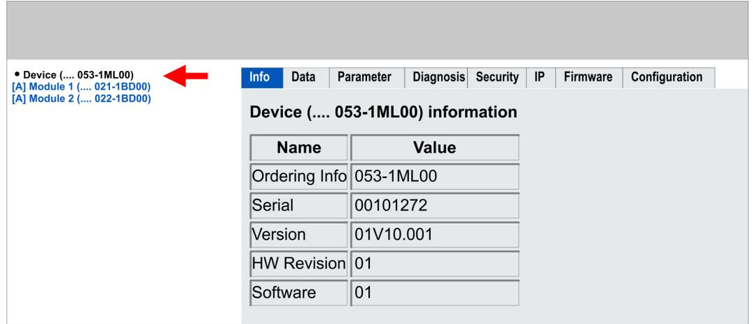
**Info** Here order number, serial number and the version of firmware and hardware of the MECHATROLINK-III coupler are listed.
