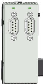
By using extension modules you can extend the interfaces of the CPU. The attachment to the CPU is made by plugging on the left side of the CPU. You can only connect one extension module to the CPU at a time.
